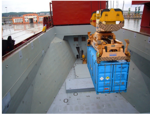
Figure 6. Loading of ISO containers with HEU fuel into vessel cargo hold
