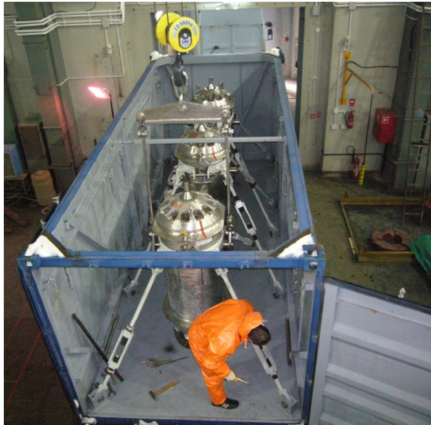
Figure 4. TUK-19 casks in ISO container
