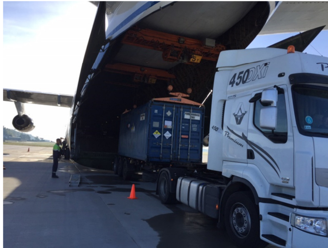
Figure 7. Loading of ISO containers with HEU fuel into An-124 cargo plane
